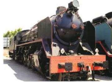
Locomotora 141F-2101 (Renfe 2101) Mikado 1953 North British Locomotive (Regne Unit) 119.500 / 166.500 kg 2.000 CV (1.742 kW) 90 / 115 km/h
