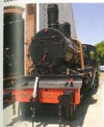
Locomotora 230-4001 (MZA 651) Compound 1901 Henschel i Maffei (Alemanya) 77.350 / 105.530 kg 1.041 CV (766 kW) 100 km/h
