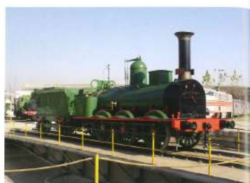
Locomotora 030-2013 (MZA 246) Mamut 1857 E. B. Wilson (Leeds, Regne Unit) 34.200 / 49.290 kg 422 CV (311 kW) 50 km/h
