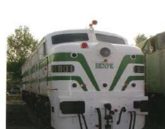
Locomotora 318-001 (Renfe 1801) 1958 ALCO i General Electric (EUA) 101.000 kg 1.457 kW 120 km/h
