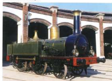
Locomotora 120-2112 (MZA 168) Martorell 1854 Sharp & Stewart (Manchester, Regne Unit) 26.333 / 34.700 kg 630 CV (464 kW) 60 km/h
