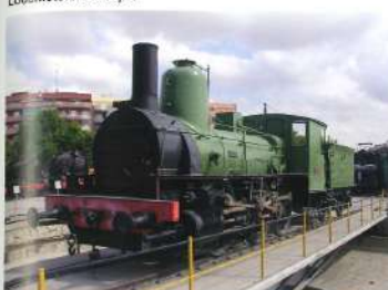
Locomotora 030-2110 (Norte 1653) Perruca 1881 Kochlin (Alemanya) 46.636 / 64.770 kg 499 CV (366 kW) 60 km/h
