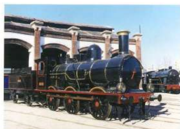
Locomotora 030-2369 (Alcantarilla - Lorca 4) 1884 Sharp & Stewart (Regne Unit) 43.600 / 61.800 kg 938 CV (691 kW) 60 km/h
