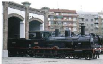
Locomotora 220-2023 (Andalucía 6) Bobadilla 1890 Beyer, Peacock & Co. (Regne Unit) 47.194 / 61.976 kg 595 CV (438 kW) 80 km
