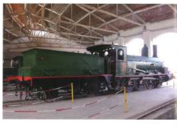
Locomotora 040-2019 (MZA 571) Vilanova 1879 Sharp & Stewart (Manchester, Regne Unit) 42.882 / 47.688 kg 835 CV (613 kW) 50 km/h
